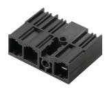
Male header with middle solder flange fastening in 10.16 pitch for 400-V IT systems according to IEC 61800-5-1. UL approval in compliance with UL840 (600 V) when using leading contact. When used together with the BUZ 10.16 IT, they comply with the expanded requirements for 5.5 mm of touch protection with IT systems (400 V relative to earth), according to IEC 61800-5-1. The middle-flange interlock feature decreases the space
