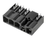
Male header with middle solder flange fastening in 10.16 pitch for 400-V IT systems according to IEC 61800-5-1. UL approval in compliance with UL840 (600 V) when using leading contact. When used together with the BUZ 10.16 IT, they comply with the expanded requirements for 5.5 mm of touch protection with IT systems (400 V relative to earth), according to IEC 61800-5-1. The middle-flange interlock feature decreases the space required by one pitch width when compared to other
