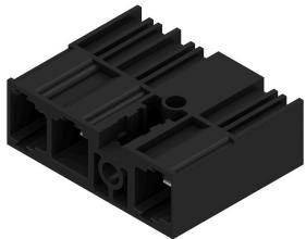
Male header with middle solder flange fastening in 10.16 pitch for 400-V IT systems according to IEC 61800-5-1. UL approval in compliance with UL840 (600 V) when using leading contact. When used together with the BUZ 10.16 IT, they comply with the expanded requirements for 5.5 mm of touch protection with IT systems (400 V relative to earth), according to IEC 61800-5-1. The middle-flange interlock feature decreases the space required by one pitch width when compared to other standard solutions.
