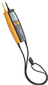
The main function of the voltage tester is to establish if voltage is present. A 2-pole voltage tester is the only approved testing instrument that fulfills the requirements of work protection regulations.
