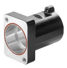
The protective housing is manufactured from seawater-resistant aluminium using pressure die casting. High standards of water and dust protection, as well as particularly high impact resistance, are the hallmarks of this housing series.
