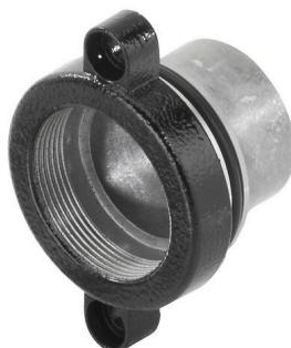
The protective housing is manufactured from seawater-resistant aluminium using pressure die casting. High standards of water and dust protection, as well as particularly high impact resistance, are the hallmarks of this housing series. A sophisticated two-stage surface coating ensures years of reliability. All screws, crimp contacts and other exterior accessory parts are made of corrosion-resistant stainless steel.
