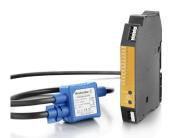
Rogowski coilA Rogowski coil is a closed air coil without a ferromagnetic core used for floating potential measurement of AC and pulse currents. Measurement with the Ragowski coil is used widely in technology, as it can be retroactively integrated without separating the primary electric circuit in existing systems. Because this method shows no saturation effect, even the smallest currents and high-frequency harmonics can be measured without loss of accuracy.
