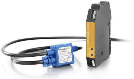
Rogowski coilA Rogowski coil is a closed air coil without a ferromagnetic core used for floating potential measurement of AC and pulse currents. Measurement with the Rogowski coil is used widely in technology, as it can be retroactively integrated without separating the primary electric circuit in existing systems. Because this method shows no saturation effect, even the smallest currents and high-frequency harmonics can be measured without loss of accuracy.
