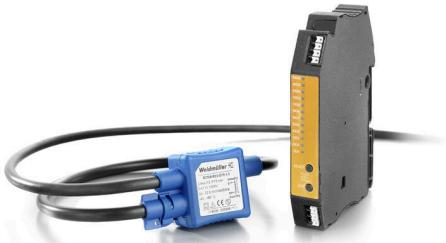
Rogowski coilA Rogowski coil is a closed air coil without a ferromagnetic core used for floating potential measurement of AC and pulse currents. Measurement with the Rogowski coil is used widely in technology, as it can be retroactively integrated without separating the primary electric circuit in existing systems. Because this method shows no saturation effect, even the smallest currents and high-frequency harmonics can be measured without loss of accuracy.
