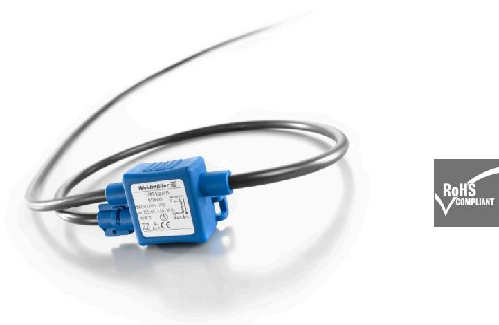
**Rogowski coil** A Rogowski coil is a closed air coil without a ferromagnetic core used for floating potential measurement of AC and pulse currents. Measurement with the Rogowski coil is used widely in technology, as it can be retroactively integrated without separating the primary electric circuit in existing systems. Because this method shows no saturation effect, even the smallest currents and high-frequency harmonics can be measured without loss of accuracy.
