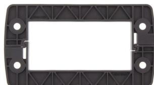
The frame, fabricated from a single piece, is quick and easy to assemble and consists of dimensionally stable, fibre-glass reinforced plastic. The captive foamed seal guarantees effective IP66 sealing in accordance with DIN EN 60529, even on painted and rough surfaces.
