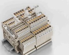
SnapMark - this tag carrier has been developed specifically for the I-series double-level terminal IDK 1.5N. The flexible pivot mechanism allows cross-connections to be easily installed or removed. It can hold four DEK 5 labelling tags or two WS 10/5 Middle connector markers.
