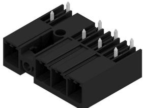
270° male header with middle flange with a 7.62 pitch. Meets the requirements of IEC 61800-5-1 and enables UL approval as per UL840 600 V. Without a female header, the mating profile guarantees minimum touch safety of >3 mm with 20 N pressure on the test finger. The automatically locking middle flange which can optionally also be screwed, reduces space requirements by one pitch width in comparison with conventional solutions.
