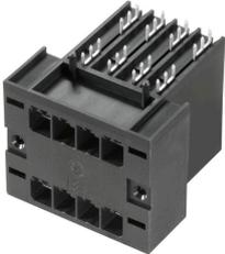
Double-row high-current, high-performance pin headers, with or without flange, for fast, tool-free locking. Optimised for "book-size modules" measuring 50mm wide and above. With integrated mounting option for mounting to the housing wall. Exceptional reliability and operational safety thanks to 100% failsafe mating profile, unique coding and optional additional screw mounting in the flange.
