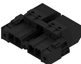
180° inverted male header with PUSH IN connection technology for field wiring in 6 mm<sup>2</sup> with 7.62 pitch as "three-flange variant" for housing passage. Suitable for housings with a max. wall thickness of 2 mm. Also perfect as a finger-safe solution for inverse voltages. Meets the requirements of UL1059 600 V class C and IEC 61800-5-1.
