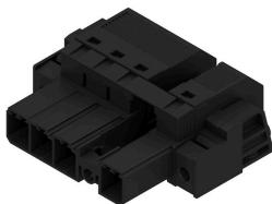
180° inverted male header with PUSH IN connection technology for field wiring in 6 mm<sup>2</sup> with 7.62 pitch as "three-flange variant" for housing passage. Suitable for housings with a max. wall thickness of 16 mm. Also perfect as a finger-safe solution for inverse voltages. Meets the requirements of UL1059 600 V class C and IEC 61800-5-1.
