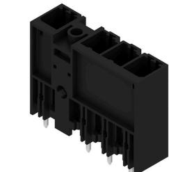
180° male header with middle flange with a 7.62 pitch. Meets the requirements of IEC 61800-5-1 and enables UL approval as per UL840 600 V. Without a female header, the mating profile guarantees minimum touch safety of >3 mm with 20 N pressure on the test finger. The automatically locking middle flange which can optionally also be screwed, reduces space requirements by one pitch width in comparison with conventional solutions. On request: available with screw flange or without flange.
