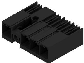
90° male header with middle flange with a 7.62 pitch. Meets the requirements of IEC 61800-5-1 and enables UL approval as per UL840 600 V. Without a female header, the mating profile guarantees minimum touch safety of >3 mm with 20 N pressure on the test finger. The automatically locking middle flange which can optionally also be screwed, reduces space requirements by one pitch width in comparison with conventional solutions.
