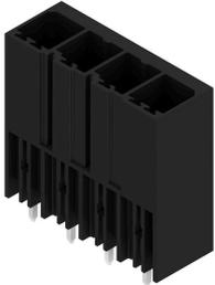
Single-row, high-performance male header for side-by-side mounting without sacrificing any poles or with patented flange for fast fixing without tools. Maximum connection and operating reliability thanks to a mating profile that prevents incorrect connection, with unique coding diversity and additional fastening in the flange. 3.5 mm pin length is optimised for lead-free wave soldering.
