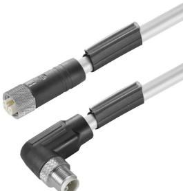
Your peripheral devices should be supplied with greater power. With our new M12 plug-in connector, more than 250 V and 2 A is possible without problems. The compact A-, K-, L-, S- and T-coded M12 plug-in connectors are designed for the transmission of up to 630 V AC or 60 V DC and 12 A.
