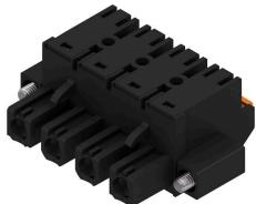
180° female header with PUSH-IN connection technology for field wiring in 2.5 mm<sup>2</sup> with a 7.62 pitch.
