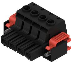
High-performance female header with the proven, 100% maintenance-free Weidmüller steel clamping yoke. Side-by-side mounting without sacrificing any poles or with patented multifunction flange for secure, fast fixing without tools. Maximum connection and operating reliability thanks to a mating profile that prevents incorrect connection, unique coding diversity, protection against incorrect wiring and 4-point silver contact.
