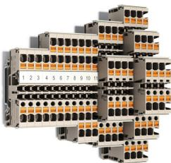
To feed through power, signal, and data is the classical requirement in electrical engineering and panel building. The insulating material, the connection system and the design of the terminal blocks are the differentiating features. A feed-through terminal block is suitable for joining and/or connecting one or more conductors. They could have one or more connection levels that are on the same potential or insulated against one another.
