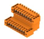
Double-level, staggered pin header for wave soldering at 3.50 mm pitch. They are available in closed and flanged versions. The male connectors provide space for labelling and can be coded.
