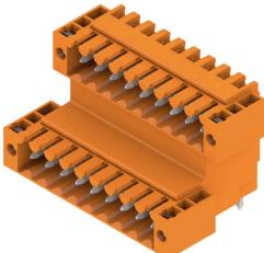
Double-level, staggered pin header for wave soldering at 3.50 mm pitch. They are available in closed and flanged versions. The male connectors provide space for labelling and can be coded.
