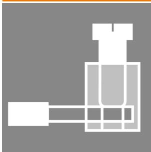
M12 plug-in connector in IP 67 available with crew or tension clamp connection
