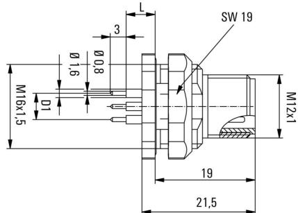
L (board-to-board distance) = 12mm D1 = 5,0 mm
