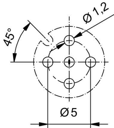
**Front panel section**
