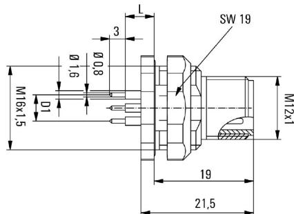
L (board-to-board distance) = 12mm D1 = 5,0 mm
