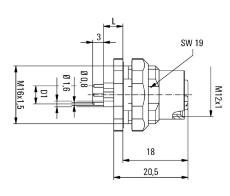
L(board-to-board distance) = 12mm D1 = 5,0 mm
