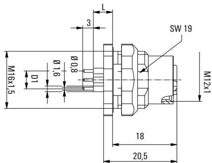
L(board-to-board distance) = 12mm D1 = 5,0 mm
