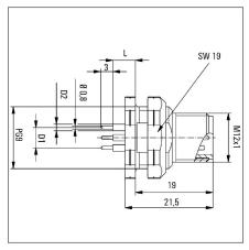
L (board-to-board distance) = 12mm D1 = 5,0 mm D2 = 1,6 mm
