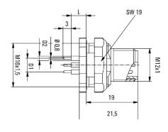
L (board-to-board distance) = 5.5mm D1 = 5,5 mm D2 = 1,4 mm
