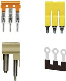
The distribution or multiplication of a potential to adjoining terminal blocks is realized via a cross-connection. Additional wiring effort can be easily avoided. Even if the poles are broken out, contact reliability in the terminal blocks is still ensured. Our portfolio offers pluggable and screwable cross-connection systems for modular terminal blocks.
