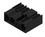
Male header with middle solder flange fastening in 10.16 pitch for 400-V IT systems according to IEC 61800-5-1. UL approval in compliance with UL840 (600 V) when using leading contact. When used together with the BUZ 10.16 IT, they comply with the expanded requirements for 5.5 mm of touch protection with IT systems (400 V relative to earth), according to IEC 61800-5-1. The middle-flange interlock feature decreases the space
