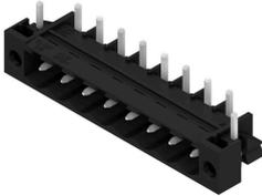
High-temperature-resistant, straight, open pin header. Packed in box or tape. On tape and with 1.5 mm solder pin, optimised for automatic assembly. 3.2 mm solder pin suitable for reflow and wave soldering. The pin headers provide space for labelling and can be coded. HC = High Current.
