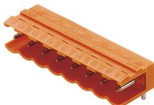
Male connectors with 90° outlet direction. The solder pin length is optimised for wave flow soldering. The pin headers provide space for labelling and can be coded.
