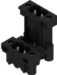
High-temperature resistant, double level, laterally offset, closed ended male header, with solder flange option. 1.5 mm solder pin suitable for reflow soldering. 3.2 mm solder pin suitable for reflow and wave soldering. The pin headers provide space for labelling and can be coded.
