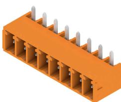
The SC pin header in 270°-outlet direction: the 270° angle exists between the plugging direction and the solder pin. The plugging direction is then parallel to the PCB. Sockets blocks, however, have an overhead plugging angle.
