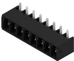
The SC-SMT pin header in 270°-outlet direction: the 270° angle exists between the plugging direction and the solder pin. The plugging is then parallel to the PCB. Sockets blocks, however, have an overhead plugging angle.
