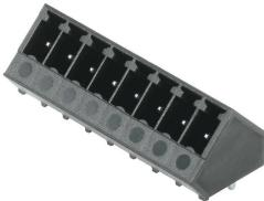
The high-temperature-resistant SC-SMT pin header with 135° wire outlet direction: the 135° angle exists between the plugging direction and the solder pin. The wire outlet direction is then diagonal or 45° to the PCB.
