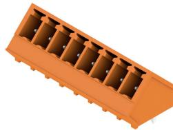
The SC pin header with 135° wire outlet direction: the 135° angle exists between the plugging direction and the solder pin. The wire outlet direction is then diagonal or 45° to the PCB.
