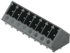
The high-temperature-resistant SC-SMT pin header with 135° wire outlet direction: the 135° angle exists between the plugging direction and the solder pin. The wire outlet direction is then diagonal or 45° to the PCB.
