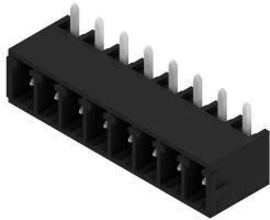
The SC-SMT pin header in 270°-outlet direction: the 270° angle exists between the plugging direction and the solder pin. The plugging direction is then parallel to the PCB. Sockets blocks, however, have an overhead plugging angle.
