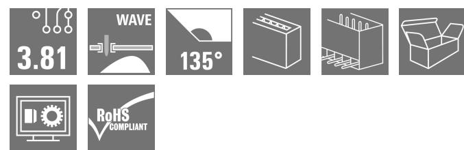
The SC pin header with 135° wire outlet direction: the 135° angle exists between the plugging direction and the solder pin. The wire outlet direction is then diagonal or 45° to the PCB.
