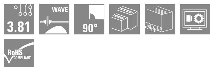
Two-tier SCD pin header for wave soldering.
