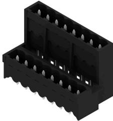
High-temperature resistant, double level, laterally offset, closed ended male header, with solder flange option. 1.5 mm solder pin suitable for reflow soldering. 3.2 mm solder pin suitable for reflow and wave soldering. The pin headers provide space for labelling and can be coded.
