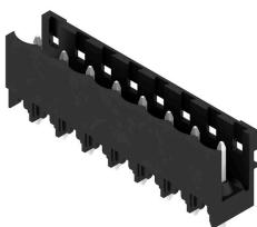
High-temperature-resistant, straight, open pin header. Packed in box or tape. On tape and with 1.5 mm solder pin, optimised for automatic assembly. 3.2 mm solder pin suitable for reflow and wave soldering. The pin headers provide space for labelling and can be coded. HC = High Current.
