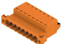
Male plug with PUSH IN wire connection and straight outlet direction, when used with BLF 5.08HC as wire-to-wire application for panel feed-through. The male plugs provide space for labelling and can be coded.
