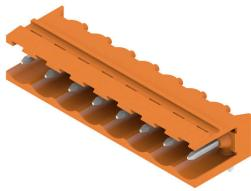
Pin headers made from glass-fibre-reinforced plastic with 90° wire outlet; optimised for wave soldering. The flange variant (F) can be screwed onto the respective counter piece or the circuit board. There is no need for an extra screw to connect the circuit board when the solder flange (LF) version is used. This also protects the solder points from mechanical strain. All pin headers can be manually coded or ordered pre-coded. HC = High Current.
