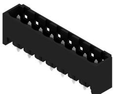
High-temperature-resistant pin header, packed in box or tape. On tape, with 1.5 mm solder pin, optimised for automatic assembly. 3.2 mm solder pin suitable for reflow and wave soldering. The pin headers provide space for labelling and can be coded. HC = High Current.
