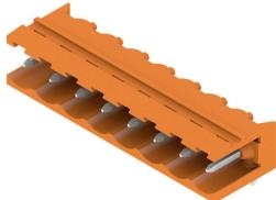
Pin headers made from glass-fibre-reinforced plastic with 90° wire outlet; optimised for wave soldering. The flange variant (F) can be screwed onto the respective counter piece or the circuit board. There is no need for an extra screw to connect the circuit board when the solder flange (LF) version is used. This also protects the solder points from mechanical strain. All pin headers can be manually coded or ordered pre-coded. HC = High Current.
