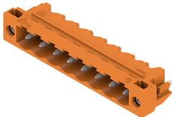
Pin headers made from glass-fibre-reinforced plastic with 90° wire outlet; optimised for wave soldering. The flange variant (F) can be screwed onto the respective counter piece or the circuit board. There is no need for an extra screw to connect the circuit board when the solder flange (LF) version is used. This also protects the solder points from mechanical strain. All pin headers can be manually coded or ordered pre-coded. HC = High Current.
