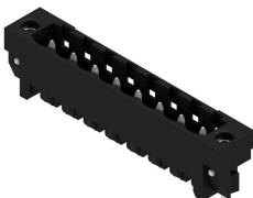
High-temperature-resistant pin header, packed in box or tape. On tape, with 1.5 mm solder pin, optimised for automatic assembly. 3.2 mm solder pin suitable for reflow and wave soldering. The pin headers provide space for labelling and can be coded. HC = High Current.
