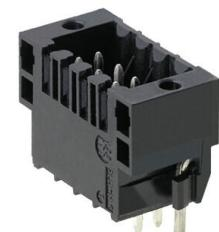
High-temperature-resistant, double-row pin header for all common soldering methods. Optimised for automatic assembly. Packed in box or tape. Solder pin 3.2 mm long, suitable for reflow and wave soldering. The male connectors provide space for labelling and can be coded.
