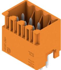
Straight, double-row pin header available in closed-sided or flange version (open-sided pin headers on request). The male headers with a pin length of 3.5mm are designed for wave soldering and are packed in a box. They can be screwed on to the PCB. The male headers provide space for labelling and can be coded.
