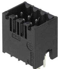
High-temperature-resistant, double-row pin header for all common soldering methods. Optimised for automatic assembly. Packed in box or tape. Solder pin 3.2 mm long, suitable for reflow and wave soldering. The male connectors provide space for labelling and can be coded.
