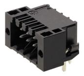
High-temperature-resistant, straight, 2-tier male connector for all common soldering methods. Optimised for automatic assembly. Packed in box or tape. 3.2 mm solder pin suitable for reflow and wave soldering. These male connectors can be labelled and coded.
