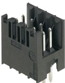
High-temperature-resistant, double-row pin header for all common soldering methods. Optimised for automatic assembly. Packed in box or tape. Solder pin 3.2 mm long, suitable for reflow and wave soldering. The male connectors provide space for labelling and can be coded.
