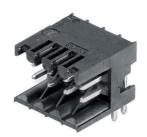
High-temperature-resistant, straight, 2-tier pin header for all common soldering methods. Optimized for automatic assembly. Packed in box or tape. 3.2 mm solder pin suitable for reflow and wave soldering. These pin headers can be labelled and coded. (Packaging in tape on request)
