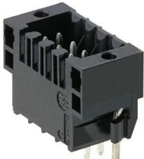
High-temperature-resistant, double-row pin header for all common soldering methods. Optimised for automatic assembly. Packed in box or tape. Solder pin 3.2 mm long, suitable for reflow and wave soldering. The male connectors provide space for labelling and can be coded.
