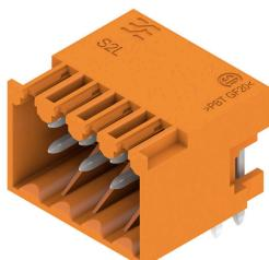
Angled, two-tier pin header available as closed-sided or with flange (open-sided pin headers on request). Pin headers with 3.5mm pins are designed for wave soldering and are packaged in a box. They can be screwed on to the PCB. The pin headers provide space for labelling and can be coded.
